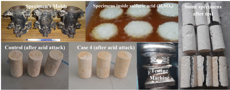
Fig. 2. Specimens' Molds; Cement Mortar Specimens (With Micro-organisms; Without Micro-organisms; Inside Acid Attack; After Acid Attack); Testing Machine and Some tested specimens.
