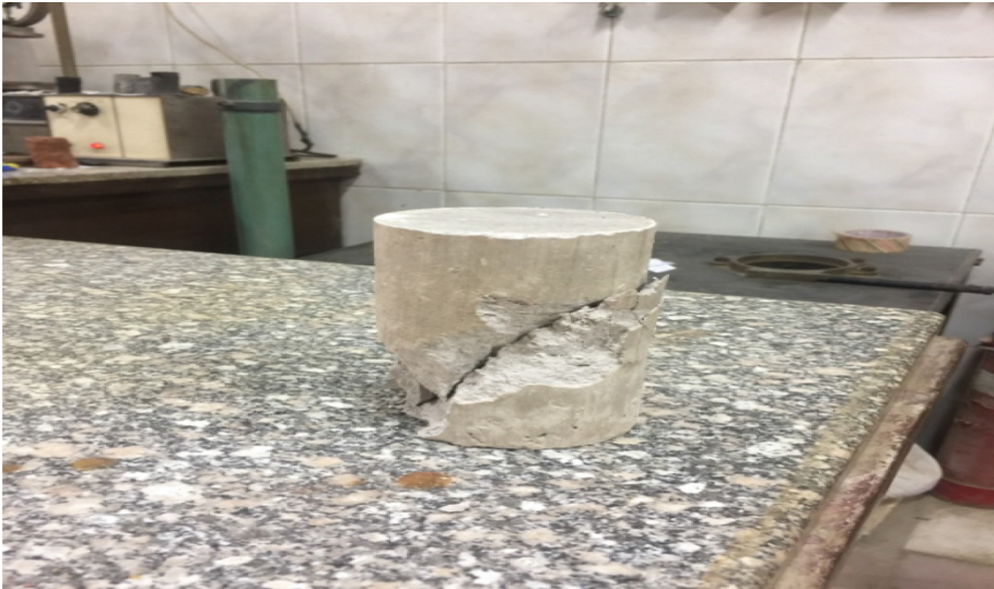
Fig. 6. Failure shapes of acceptance tested samples
