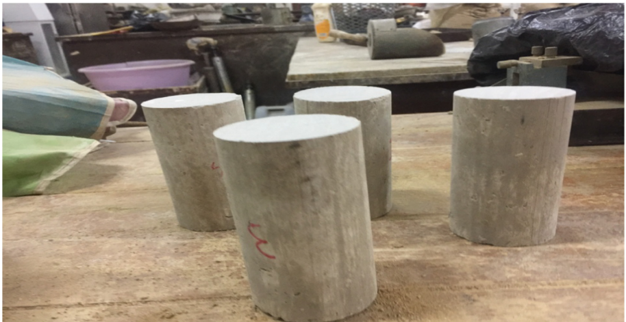
Fig. 4. Acceptation tested samples of CKD after drying for 7 days
