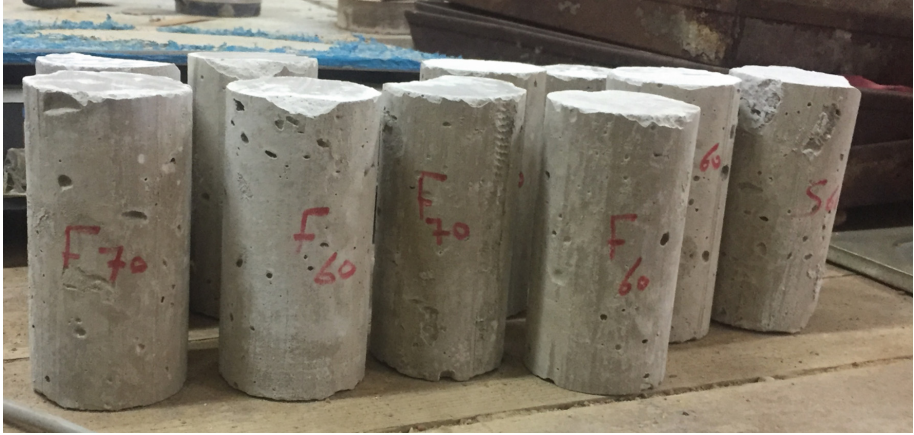
Fig. 3. Samples of CKD after drying for 7 days before rejecting the bad samples
